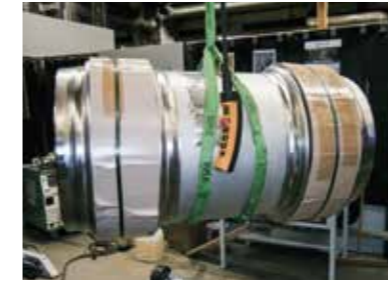
Cleaned with osmotic water, the expansion joint is now ready for dispatch.
